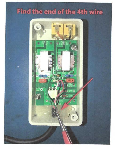
After exposing the fourth wire, make a jumper from the fourth wire to PTT HI on the board.
